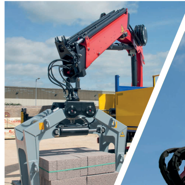
HYDRAULIC SUPPLY to auxiliary equipment
