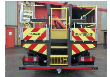
Stepped and gated rear access on a pole erection, street lighting vehicle.
