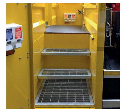
Low entry non slip access steps to body with lighting and full height lockable door.
