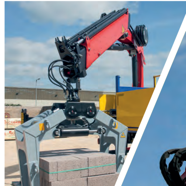
HYDRAULIC SUPPLY to auxiliary equipment
