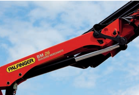
SINGLE LINK PLUS a 15 degree reverse linkage system
